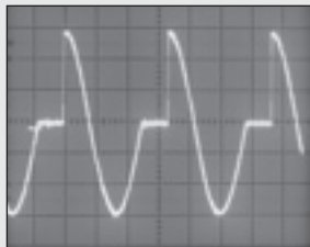
Sine wave with first quarter (0° - 90°) at 0 volts
