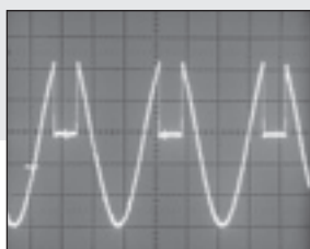
Sine wave with the positive halfcycle clipped at 0V from 50° - 130°
