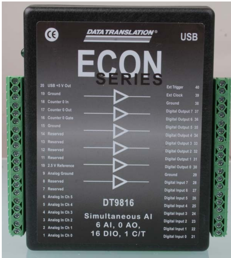
Figure 5: Screw Terminals on the DT9816, DT9816-A, and DT9816-S Modules
